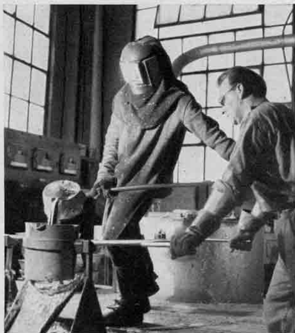
Clad in a fireproof suit, heavy metal shoes, and a helmet that looks like the headpiece of a deep-sea diver, a worker at the Martin plant near Baltimore pours molten metal to be used for die-casting. This is a little-known phase of Martin's job of filling defense orders for aircraft that run into nine figures
